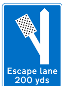
817-2L Dis Escape lane ahead for vehicles unable to stop on a steep hill (bespoke)
