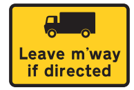
832-3 Goods vehicles may be directed to leave the motorway at the junction ahead
