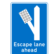
817-2L Escape lane ahead for vehicles unable to stop on a steep hill (bespoke)
