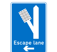
817-2LL Escape lane ahead for vehicles unable to stop on a steep hill (bespoke)
