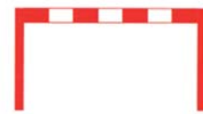
Traffic barrier ('Lane closed' sign)
